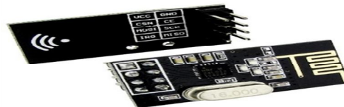
nRF24L01+2.4GHZ WIRELESS TRANSCEIVER
